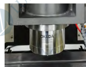
10000转主轴 10000 RPM spindle
